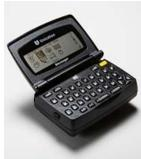
**The Unication M90** offers the latest in advanced 2Way messaging features. Small and easy to use, the M90 includes a full 39 key QWERTY keyboard, an 8-line to 5-line display zoom, and 4 way navigation keys to provide fast, 2-Way messaging. A PC serial cable is included so you can back up your data.
