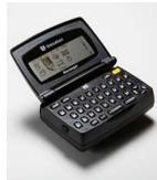
**The Unication M90** offers the latest in advanced 2Way messaging features. Small and easy to use, the M90 includes a full 39 key QWERTY keyboard, an 8-line to 5-line display zoom, and 4 way navigation keys to provide fast, 2-Way messaging. A PC serial cable is included so you can back up your data.
